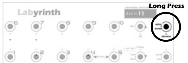
5) Use UP and DOWN buttons to select the bank where to save the new patch. Use 1 to 10 button to choose in which memory location store your preset. Simply press “ENTER” button to confirm. “COMPLETE” will appear on the display to confirm the saving of the preset in the pedalboard memory.
