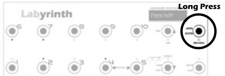
4) Again, press and hold the “Menu/Enter/SB-MEM” button until “Write to” appears on the display.
