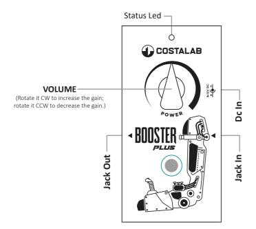
But having a range of clean boost that goes from 0 to +26db, the Costalab Booster, can be also used in the effect loop as an attenuator for loud tube amps.
